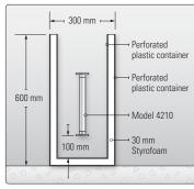
• "No stress-strain" enclosure using the Model 4210.
