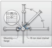
Front view of a Model 4210 strain gage rosette configuration. Inset shows rosette fixture (enlarged for detail).
