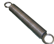
WNS / EDWARDS Treadle Guillotine Springs. Overall Length: 14". Loops: 2" Diameter. Springs: Outside Diameter: 2". Wire: 3/4". (GS14/6.3)
