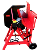
WNS Log Saw. Blade: 502mm (20"). Bore: 30mm. Cut Length: 250mm-1000mm. Speed: 2800 RPM. 240v, 50Hz, Single Phase. (LS502)
