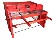
WNS Cast Treadle Guillotine. 1320mm x 1.5mm Capacity. c/w Front Support Arms, Back Stop & Rear Guard. (TG1320C)
