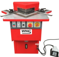
WNS Hydraulic Corner Notcher. 200mm x 200mm x 4.0mm Capacity. Cutting Angle: 90°. Motor: 3kW. 40 Strokes/min. 415v, 3 Phase. (HCN200)
