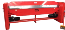
WNS Power Box & Pan Folder. 2520mm x 1.0mm Capacity. 415v, 3 Phase. (PBPF2520)
