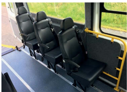
Semi-high back seat, trimmed in vinyl, trimmed headrest, armrest
