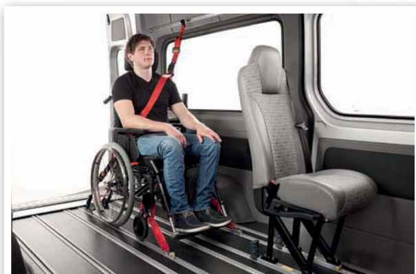
A wheelchair and user in situ, safely secured
