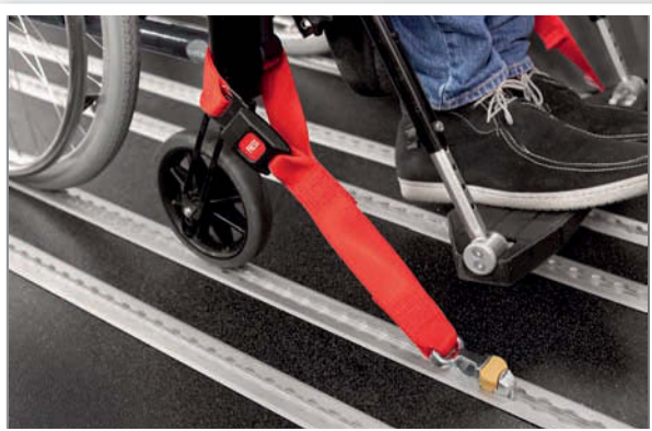
The front webbing straps are fixed, and secure the wheelchair
