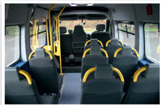
Semi-high back seat, trimmed in cloth and vinyl, twin grab headrest
