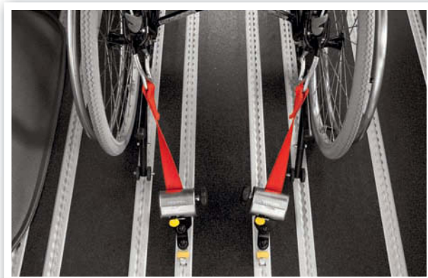
The retractable rear cassette fixing ensures the wheelchair is 'braced' against the front fixings
