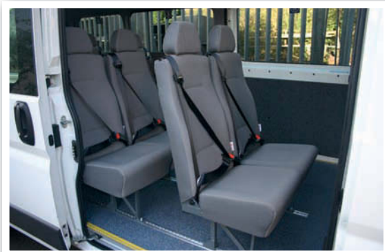
Semi-high back seat, trimmed in vinyl, trimmed headrest
