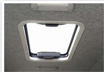
Coach style roof vents provide extra light as well as fresh air
