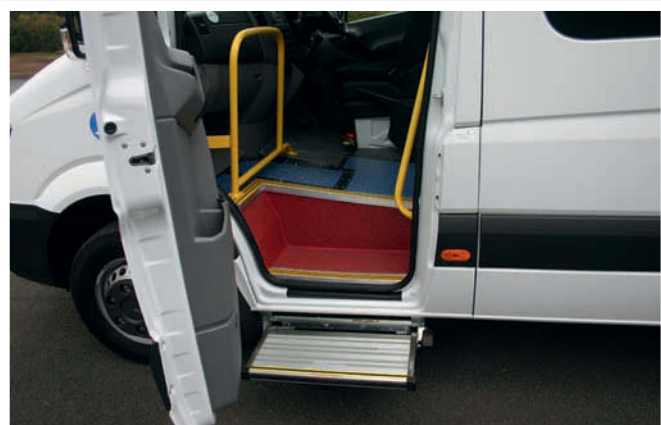
Flush folding three-step entry with vertical and half-height rail and modesty screen
