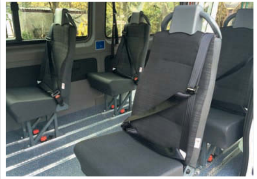
Semi-high back seat, trimmed in cloth and vinyl, twin grab headrest
