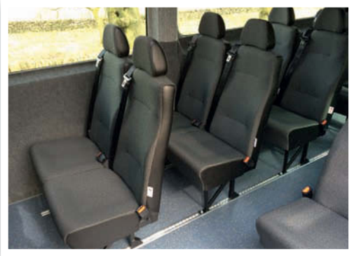
Semi-high back seat, trimmed in cloth and vinyl, trimmed headrest
