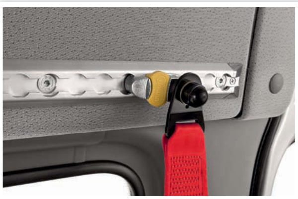
Third-point fixings in the cant rail are mandatory on M1 category vehicles
