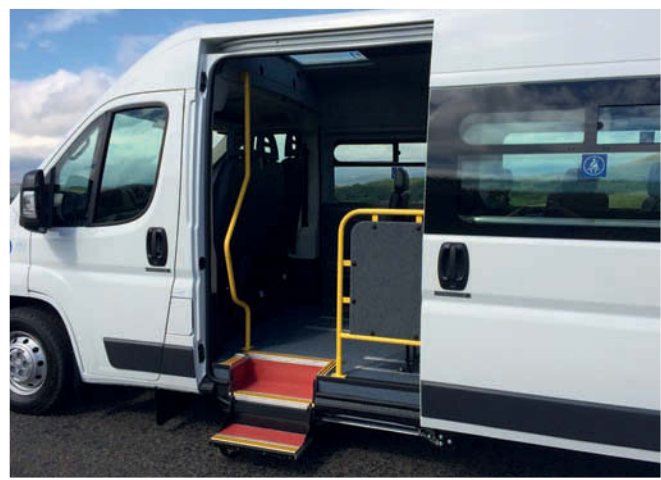
Flush folding three-step entry with vertical and half-height rail and modesty screen
