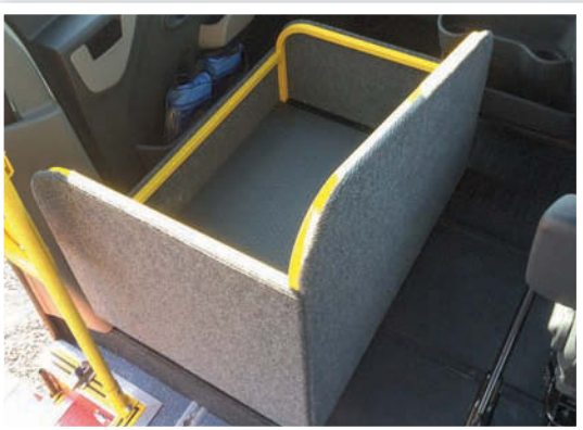
A stowage pen in the nearside cab is popular for accessible vehicles
