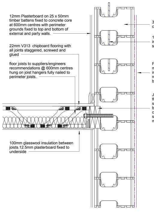
350mm wide izodom insulated concrete formwork
