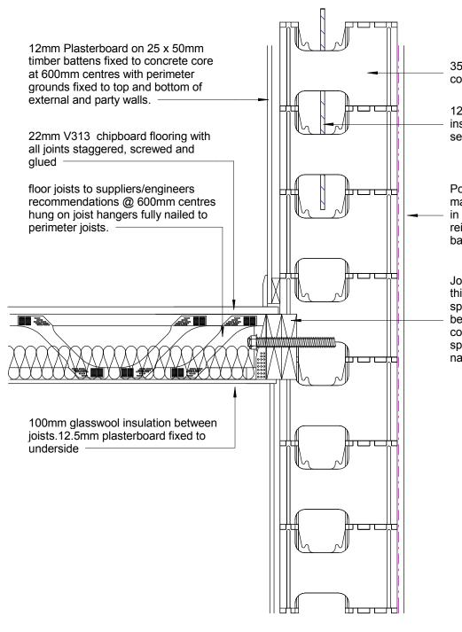
350mm wide izodom insulated concrete formwork
