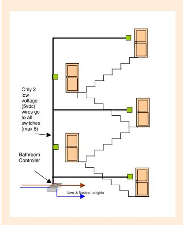
The controller has a switched output using a relay rated at 500W. and will operate all types of lighting.
