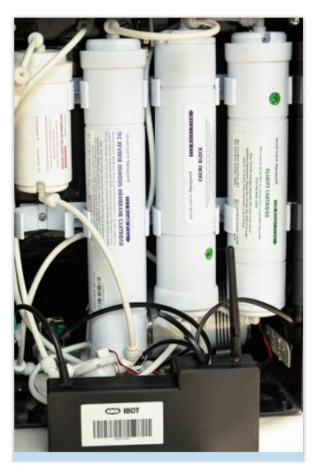
The box consisting of assembly of the iQu, Base Board and power adapter was installed inside the purifier. Special attention is paid to fitment of the adapter-PCB box so that all criteria of the client related to robustness of physical design are satisfied.
