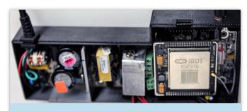
The electronics assembly comprising iQu and Base Board were integrated with the power adapter that powers the pump as well as iQu + Base Board assembly. These components collectively were installed inside a single box (again designed for the purpose). The box itself went through multiple iterations of design for attributes such as placement, fitment, and Electromagnetic Interference (EMI).
