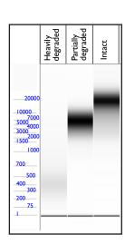
Human genomic DNA run on the Fragment Analyzer $^{\text{M}}$ , showing heavily degraded, partially degraded and intact samples. Despite the presence of heavily degraded material, the ultra fast Lower Marker (set to 1 bp) migrates quickly enough to provide successful analysis.
