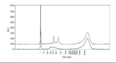
The **Fragment Analyzer**<sup>™</sup> automates both separation and subsequent analysis of gDNA. Its parallel capillary electrophoresis platform allows analysis of 11 or 95 samples with 1 ladder per run. One instrument analyzes both quality and quantity, thus greatly reducing manual lab work.
