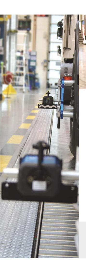
The actual measurement starts as the operator clicks the OK-button on one of the cameras, to indicate that the equipment is in place on the vehicle. The software calculates the parallelism of the front axle, using the main driven axle as the reference axle.
