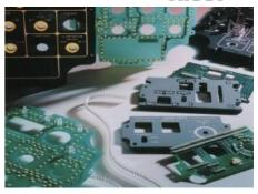
The choice of LED's in a Surface Mount configuration enables panels for aerospace and military applications to be manufactured in accordance with the dimensional and other requirements of SAE AS7788 (Formally MIL-P-7788F) for Type VII panels and other major national and corporate specifications.
