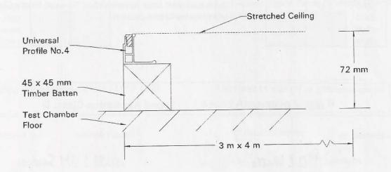
Sound Absorption Coefficient according to EN ISO 354:2003
