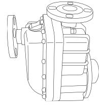
3. Remove the three hex socket cap head bolts that secure the rear casing support to the rear casing.
