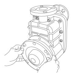
6. Remove the remaining nuts securing the front and rear cases and separate.
