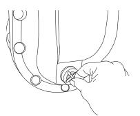
2. Next, loosen the four hex head bolts on the motor bracket to remove the pump head from the motor.
