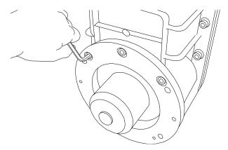
4. Remove all cover caps and the five nuts securing the front casing. At this point any remaining liquid can be drained from the pump.
