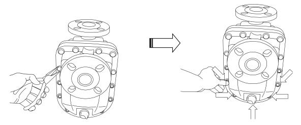
5. Separate the rear casing support, rear casing and impeller + magnet capsule unit at one time from the rear case. Note, magnet capsule should be kept free of all metal chips. Store in a clean area.
