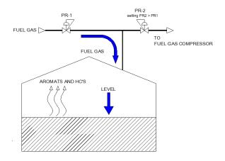
By using a fuel gas based blanketing system the composition of the returned fuel gas will be subject to rapid changes upon the filling process of the tank. The amount of VOC's in the headspace of the tank will depend on pressure, temperature and medium stored in the tank.
