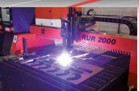
...Not quite, but the KERF high definition plasma cutting machine with UltraSharp technology produces what is accepted by many as being of a laser quality.
