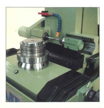
The use of special electroplated diamond grinding wheels allows the grinding of ribs with different forms and inclinations.
