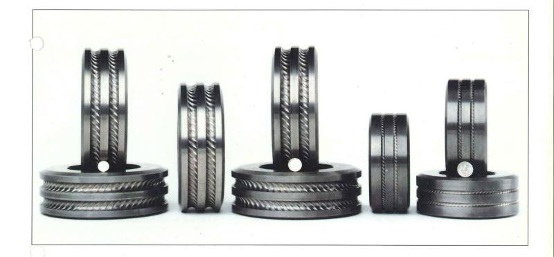
The AT810E is equipped with special diamond grinding wheels that permit the machining of the same rolls used for the production of wire rod (WC 80-85%, CO 15-20%). The use of rolls with a lower level of cobalt can lead to an increase of up to 30% in the groove life of the roll thus, reducing the quantity of rolls consumed per ton produced and the mill down time for changing rolls.
