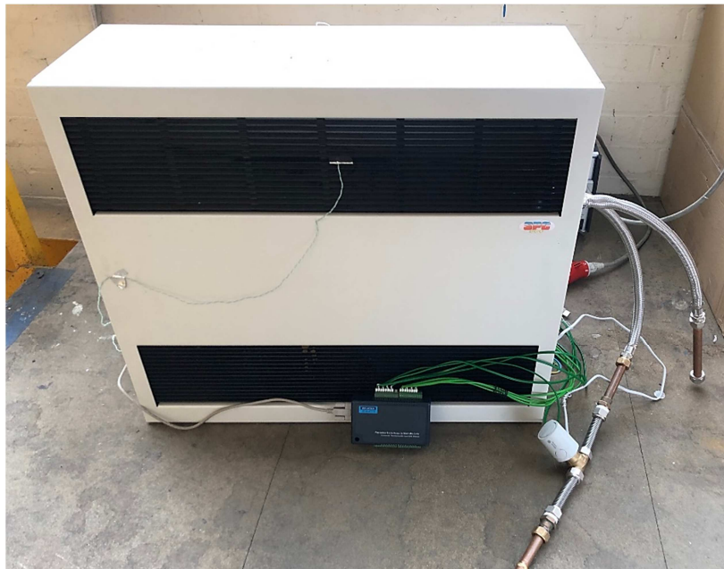
Figure 3. Test piece showing thermocouples and valve/actuator
