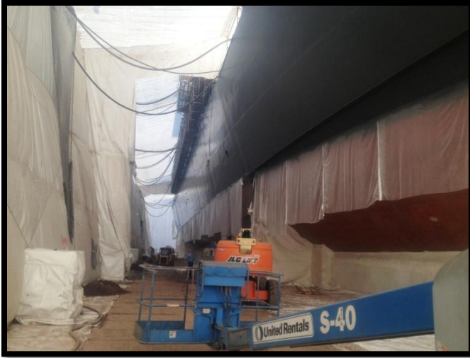
Primer application completed and YVK assures a complete sound primer coat is in place by checking for holidays prior to top coat application.
