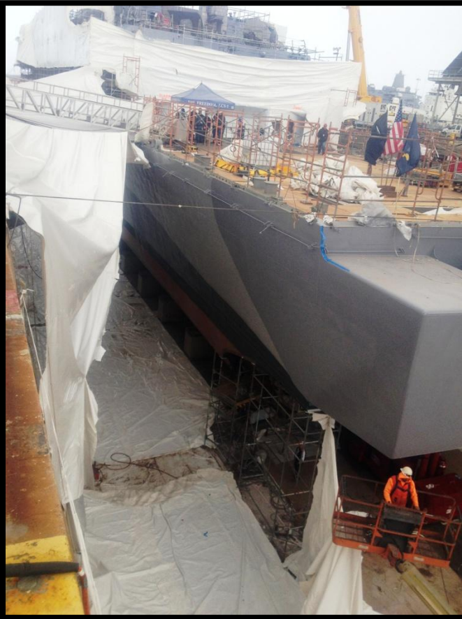
Polysiloxane camouflage paint scheme completed and tear down process begins.
