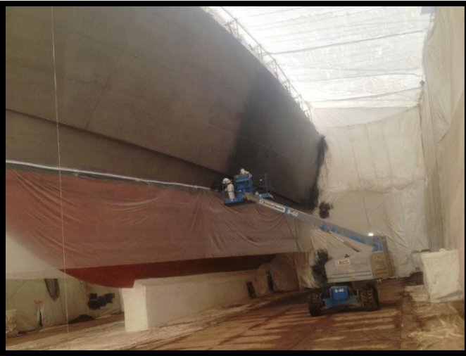
Steel & Aluminum substrates were abrasive blasted (Garnet & Copper Slag) and primed with epoxy.
