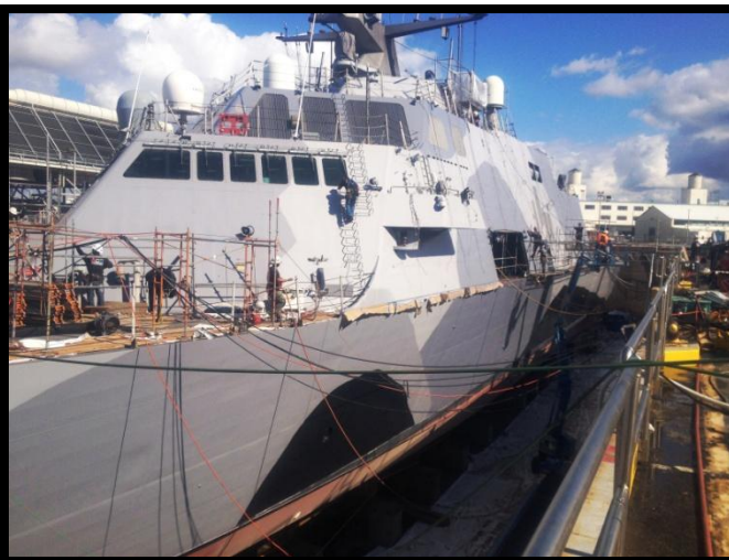
Removal of all scaffolding and cleaning of graving dock prior to undocking.
