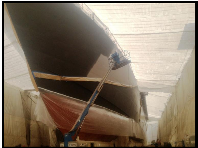
Primer application completed and YVK assures a complete sound primer coat is in place by checking for holidays prior to top coat application.
