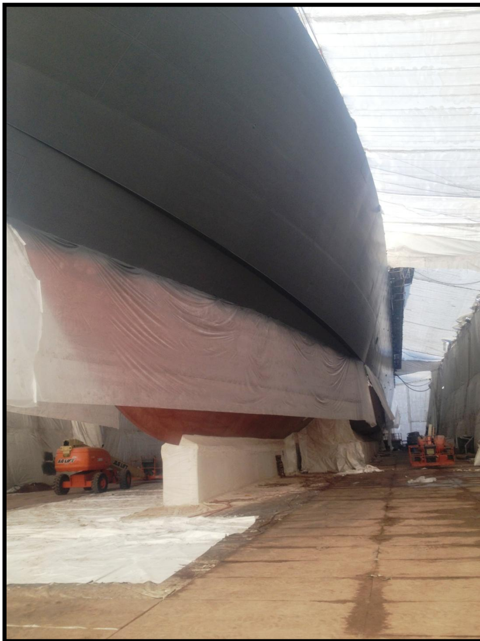
Steel & Aluminum substrates were abrasive blasted (Garnet & Copper Slag) and primed with epoxy.
