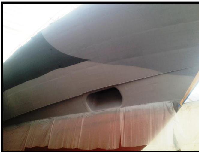
Black Polysiloxane is applied near exhaust openings so that exhaust stains don't stand out.
