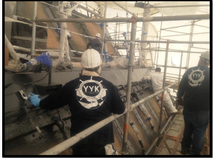
Primer application completed and YVK assures a complete sound primer coat is in place by checking for holidays prior to top coat application.
