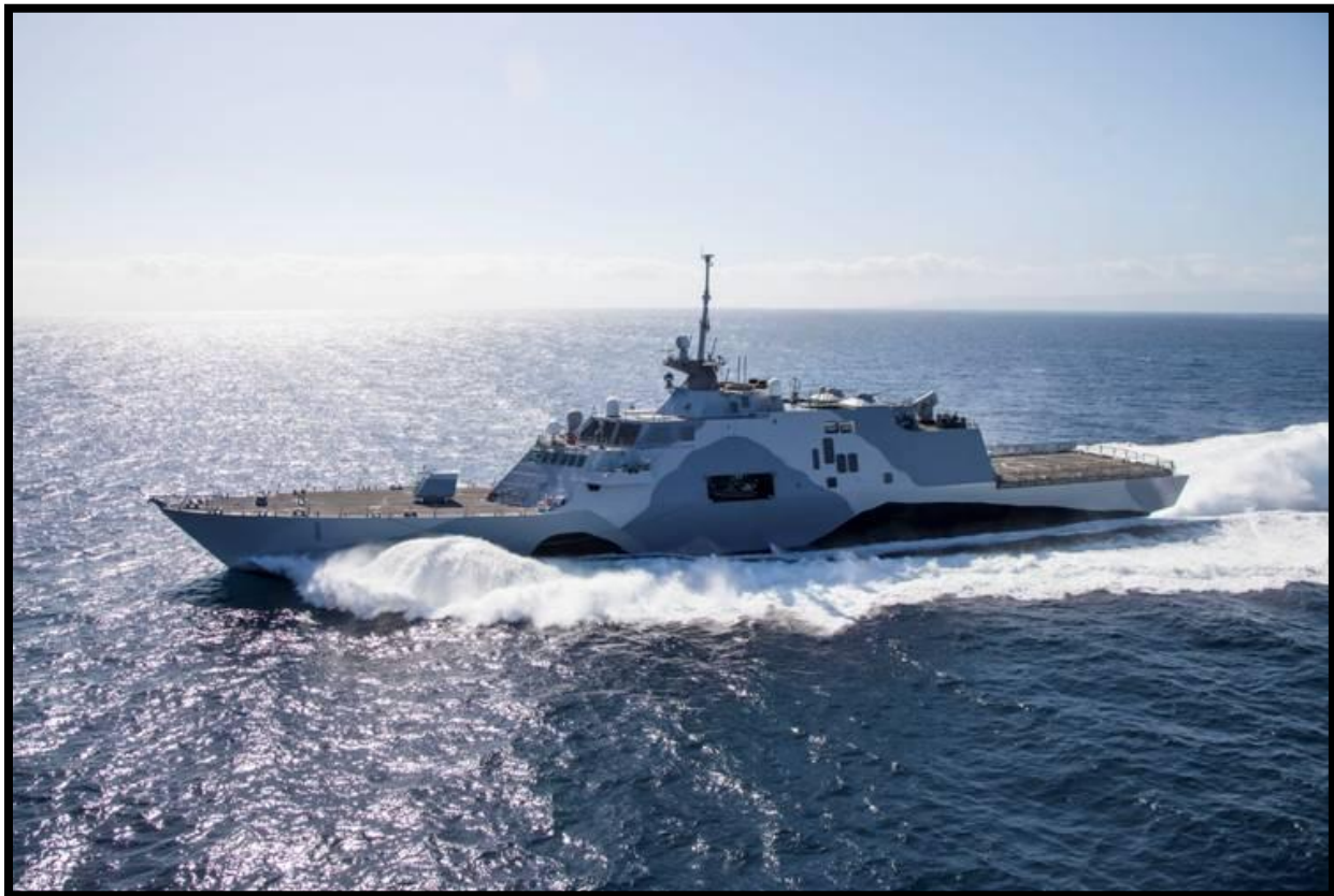
After Preservation (New Polysiloxane Camouflage Paint Scheme)
