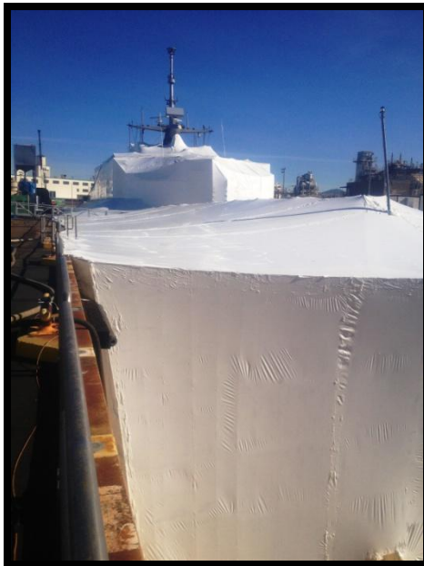
Encapsulation was completed & ready for surface preparation. The encapsulation was erected to a weather resistant degree due to the upcoming rain days which had been forecasted during the vessels availability.
