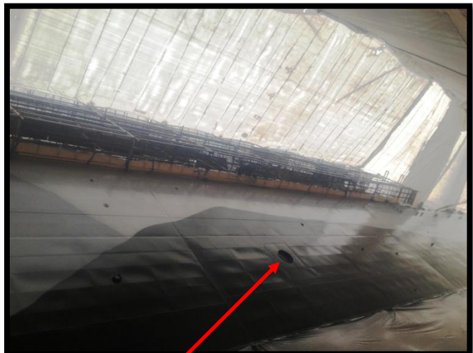
Black Polysiloxane is applied near exhaust openings so that exhaust stains don't stand out.
