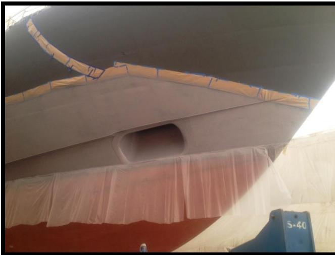
Application of Polysiloxane camouflage paint scheme begins.
