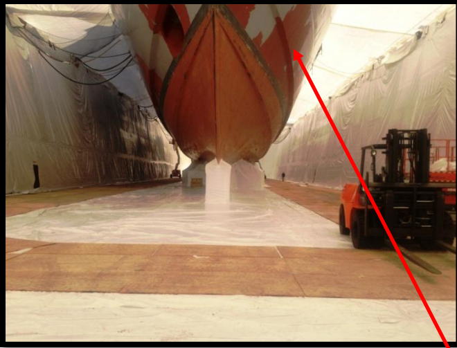
Encapsulation continues. Note existing coating failure areas.
