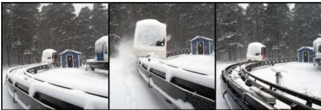
Figure 11. Vehicle clearing its way in severe ice and snow at 5m/s.
