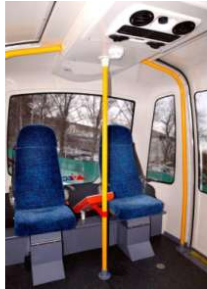
Figure 5. Vehicle interior with display panel between individual seats and roof-mounted ventilation unit.
