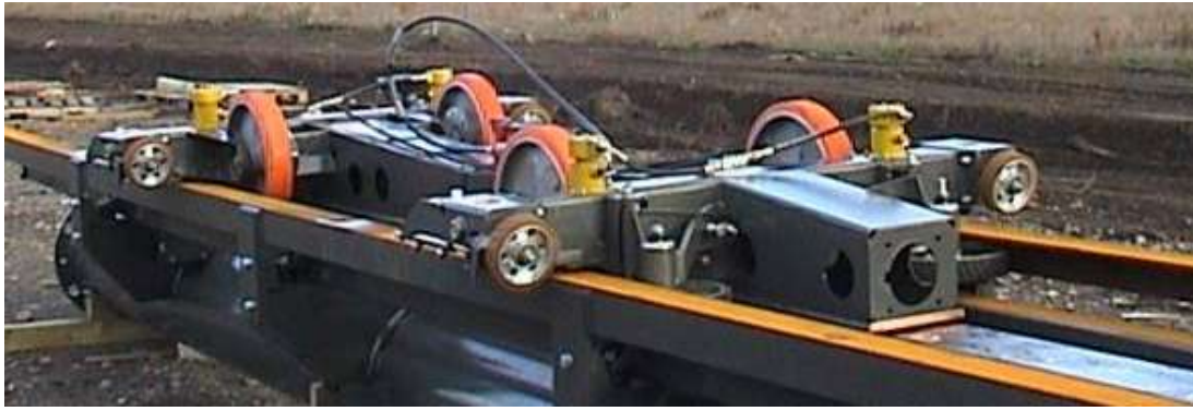
Figure 6. First chassis tested for clearance on a section of track.
