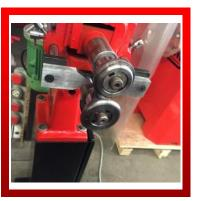
**WNS** POWER SWAGERS (PS215, PS215V, PS215sp, PS215spV) are principally used for Swaging, Beading, Wiring, Crimping and Forming of sheet metal. The Power Swager has a 215mm (8.5") Throat and can accommodate mild steel sheet up to 1.2mm thick. This machine comes complete with 6 Sets of Rolls, Forward & Reverse foot pedal and potentiometer speed control.
