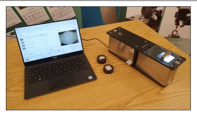
A self contained system for weld examination, recording and analysis. With built in 5MP colour camera, unique optics, inbuilt LED illuminator and linked directly to the Zeiss ZEN innovative software allows the capture, recording, measurement and reporting of your weld samples.
