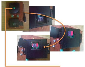
Test proposed location for range - press the phone unit fixed radio button and your assistant should see the small red LED in the cabinet flash quickly. The gate will not operate until the unit is tuned in. See 3.2 for tuning in.
