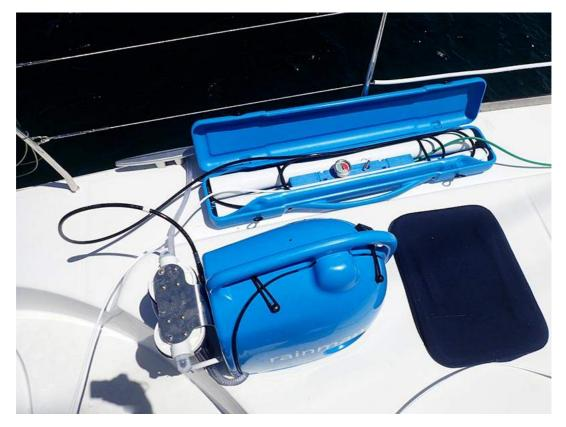
The system that *Gary* and *Marie* own has a very high output. This dual-membrane watermaker is rated to produce 100-140 lph (23-32 gph). When looking through their literature, I also read that *Rainman* offers a compact version that produces 50-70 lph, apparently good for those who have less storage room on their boats, and also an "economy" single-membrane unit, also designed to produce 50-70 lph.
