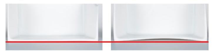
Because pressure-cooled rotomolding chills both the outside and inside of parts simultaneously, shrinkage rates are consistent, which reduces warpage. On the left is a part produced with Ripple Engineering's technology, while the part on the right, made of the same material and produced on the same tool, was cooled using the traditional method (on the outside only). The latter part exhibits significantly more warpage. Courtesy of Ripple Engineering
