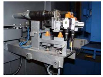
redirection of the trays with pusher and transversal pusher, are implemented in turnable way and can be adjusted in the setting operation with opened assembly door. This permits a precise and fast identification of the final position of the trays during assembling and putting into operation phase. 746 valid for the building of furnaces.
