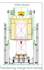
In order to protect the furnace chamber against unwanted penetration of atmospheric oxygen during the charging processes, the charge is transferred at the furnace inlet from below.
