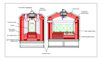
The thermal insulation consists of light-weight refractory bricks with the hearth substructure and at the side panels. The furnace cover is implemented with ceramic fibre isolation, alternatively a vault lining is also possible. In the range of charge transport SiC rails, resistant to friction, are used.
