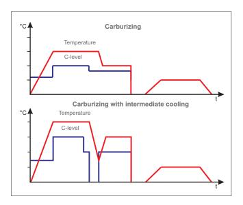
For distortion-sensitive press hardening pieces there is also the possibility of cooling them down slowly after gas carburizing in a gas cooling sluice.
