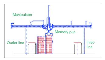
The system is controlled completely automatically via the PLC of the plant.
