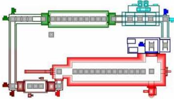
4.1 Single-lined pusher type furnace plant for carbonitriding
