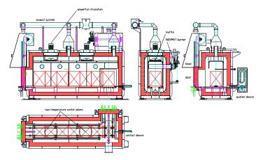
minimize the components distorsion and/or to activate the component surface for optimal carburizing results. The working temperature amounts to 400 - 480 °C (in special cases up to 600°C). Heating mostly is done by open heated gas burners, which ensure a uniform heating up of the charge, together with strengthened circulation aggregates and air guiding muffles.
