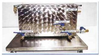
The separator works according to the physical principles of the gravitation (the force of gravity) and the coalescence (flowing together of droplets). Particles with small density ascend, heavy particles sink downward. Small droplets store themselves together to larger droplets by the coalescence principle and can be separated afterwards.
