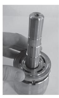
13. Position the port plate over the guide pin. IMPORTANT: Make sure that the guide pin is located in the locating hole in the port plate.
