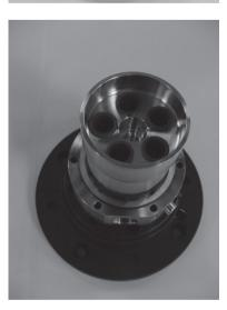
7. Remove the cylinder barrel.
