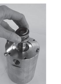
19. Replace the O-ring on the SAE flange.
