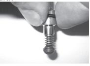
Mount flushing valve by pressing it into the hole.
