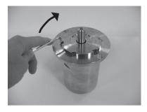
21. Tighten the screws to a torque of  $12 \pm 3$  Nm.
