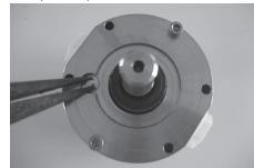
Assemble the new flushing valve, or replaced parts that are worn (shoulders)
