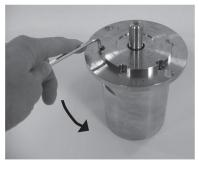
2. Wet the shaft and shaft seal with clean (filtered) soap-water. Gently lever the shaft seal assembly free using 2 screwdrivers.
