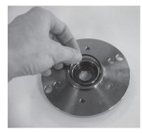
20. Lubricate the threads on the 4 screws with grease and screw them into the pump and tighten by hand. Use Molykote D paste from Dow Corning or Klüber UH1 84-201 from Klüber lubrication.
