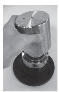
6. Remove the pistons, retaining plate, retaining ball, spring guide and spring from the cylinder barrel.
