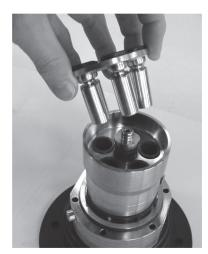
16. Position the housing on the port flange and over the guide pin.
