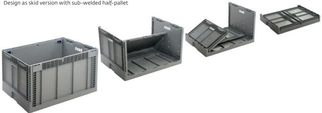
External dimensions: 800 x 600 x 465 mm Internal dimensions base: 760 x 560 x 450 mm Height collapsed: 120 mm Stacking height: 452 mm Usable int. height in stack: 425 mm Volume: 185 litres Weight: 6.9 kg
