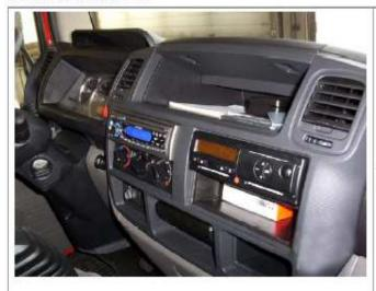
DTCO installation in the second radio compartment.
