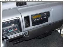
After removing the shelf compartment, the recess must be adapted to the mounting frame
