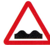
UNEVEN ROAD AHEAD P-556
