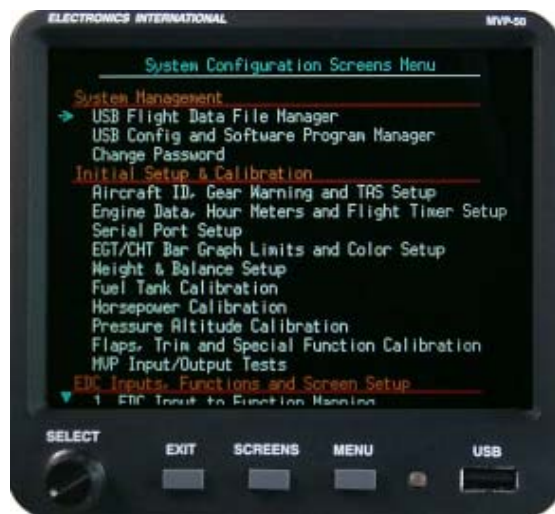
System Configuration Screens
