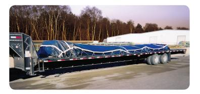
The tarps are made of Heavy-Duty Waterproof Vinyl Coated Nylon Canvas and have been field-proven on some of the harshest environments on earth. All of the tarp's seams are heat-sealed which provides superior durability as compared to sewn seams.
