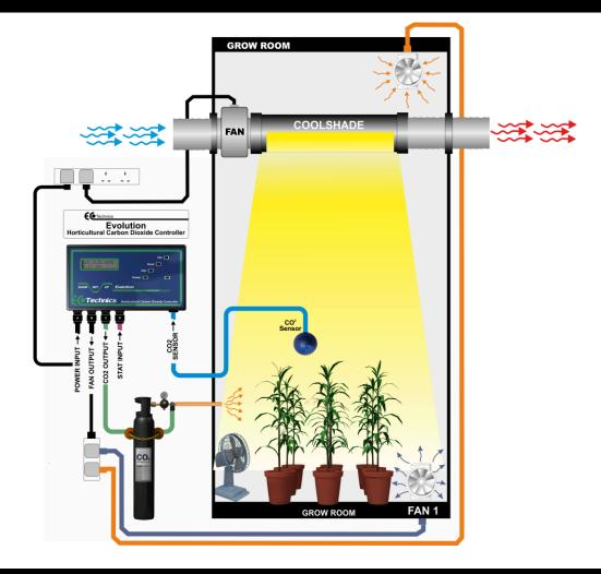
**Evolution Carbon Dioxide and Fan Speed Controllers (CoolShade)**
