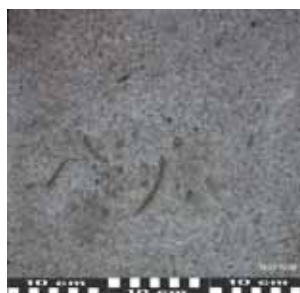
Typical Pavement Grime on a Granite surface
