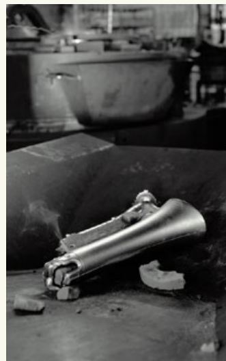
◀ The start of an Axor Massaud mixer: a raw and inconspicuous brass bar, the raw material melts in the furnace at almost 1,000 degrees. The liquid metal now takes on its typical form.
