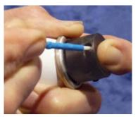
3) Dampen (do not saturate) the end of the CleanStixx™ with Sticklers™ Fiber Optic Splice and Connector Cleaner
