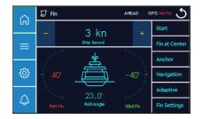
Operate stabilizers in At-Anchor mode while throttle is engaged at low speed.
