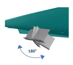
FLIP allows Stabilis Electra to rotate fins by 180° while at anchor.
