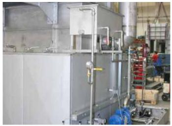
Fig.9 - Rear view chamber submersion spray cleaning unit with coalescence oil separator
