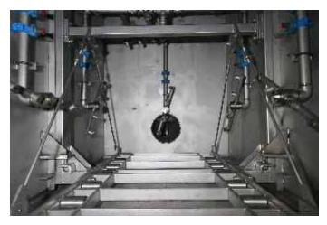
Fig.5 - Charge room chamber submersion spray unit
