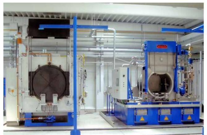
Flexiclean with 3 medium tanks integrated into a chamber furnace nitriding line
