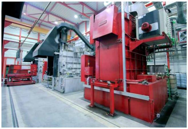
Chamber submersion spray unit with vapor vent condenser drying
