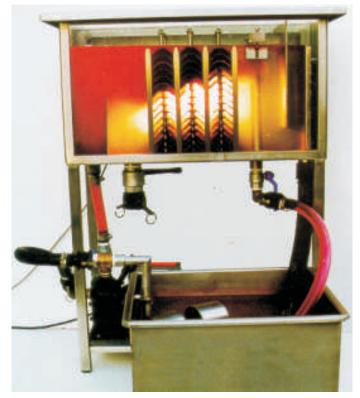
Fig.8 - 3-phase separator (interior view)
