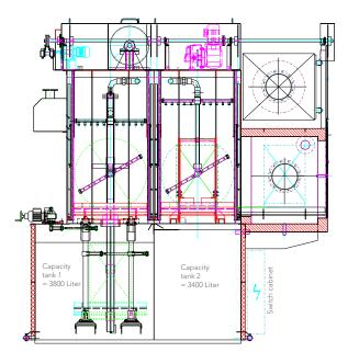
Fig.6 - Continuous submersion spray cleaning unit
