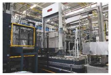
Fig.13 Flexiclean<sup>®</sup> continuous cleaning unit integrated into a pusher type gas carburizing plant
