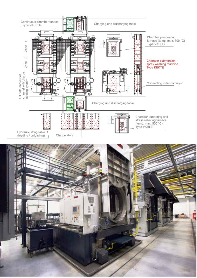
Fig.14 - Flexiclean<sup>®</sup> integrated in a double-chamber furnce line
