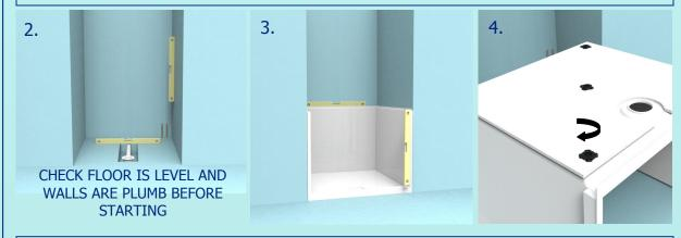
Place the tray section of the Envirotec Bathing shower in position and check for level along both walls (3). Also check that all feet are in contact with the ground (the tray should feel solid with no "spring" when tested). If adjustment is required, carefully turn the tray over using a soft blanket on the floor as protection and adjust the feet until correct floor contact is achieved (4).
