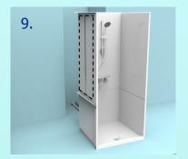
Lift the Envirotec Bathing Shower Enclosure back into the corner and mark through the pre drilled holes in the edges as shown. Drill and install suitable wall plugs according to the wall type (10). Lift the Envirotec Bathing Shower Enclosure back into its final position, connecting the water (and electrical) supply while doing so (11). Flexi pipes should be used for the water connections.
