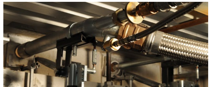
3. gas connection - inside nozzle 4. control wheel - inner nozzle position 5. gas connection - outside nozzle 6. gas nozzle - outside 7. gas nozzle - inside
