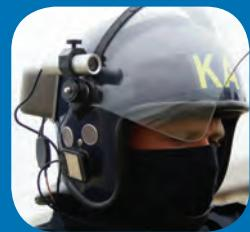
Front line, video surveillance utilising helmet mounted antennas
