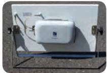
The FPA15-1.6L/1535 panel antenna can be used to operate the Thuraya IP unit at its maximum data rate.
