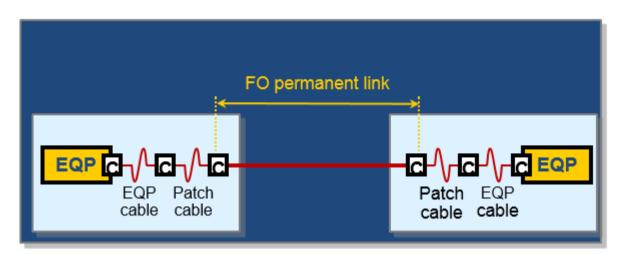
Sample of Permanent Link (EQP=equipment, C=connection)
