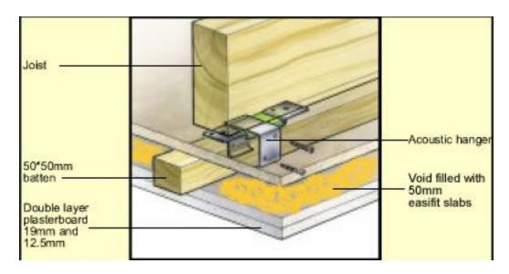
**Please note**: hangers actually run the battens perpendicular to the joists not parallel as shown in the above diagram.
