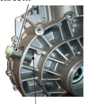
Remove Screw M18 and plate before sensor mounting!
