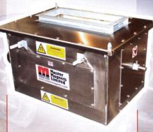
For use in high volume separation and where the product is to be kept free from external contamination or where dust may be given off during processing. Totally enclosed drum magnets allow material to flow directly over the surface of the rotating drum. Ferrous contaminants adhere to the drum surface until they are discharged behind the centre line, whilst non-metallic product free-falls at its normal trajectory.
