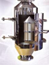
Designed for gravity feed and pressurised pipeline systems, the bullet magnet allows material to flow directly over an internal conical-shaped magnet system. The magnetic system is mounted to the quick-release doors for easy cleaning.
