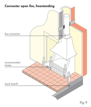
Freestanding convector fires (Fig.9 and 10) heat a larger volume of air by convection than inset fires. They are usually vented directly to the chimney with a flue connector.
