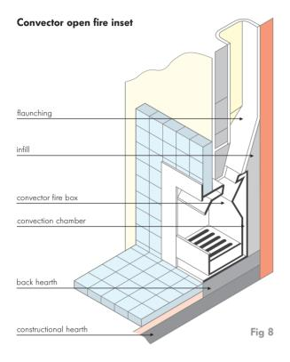
Illustrated in Fig. 8 is a double skinned firebox inset into the chimney breast to replace the usual British Standard Fireback. This type of appliance can give outputs ranging from 2.9 to 6.6kW while providing radiant and convected heat. These fires are useful in larger rooms where convected air heats a larger volume.
