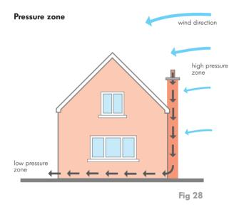
Fig. 28 shows a chimney sited in the line of the prevailing wind, with a taller object, house, roof, tree or nearby hill behind the chimney terminal. This can cause a pressure zone and puffing or continuous fume emission when the wind is blowing.
