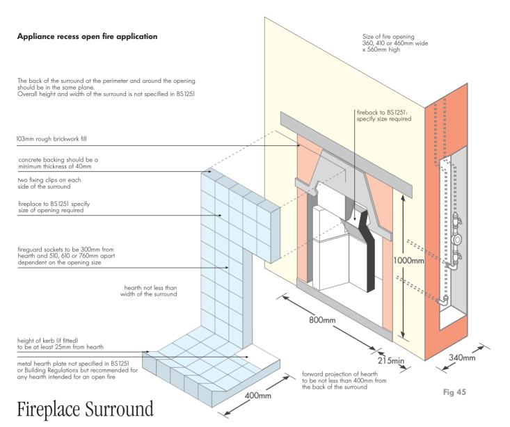
The fireplace surround and hearth illustrated above (Fig.45) is the type produced by the slabbing process and which forms the basis of the BS1251 specification. This type constitutes the major type of British fireplace in production at present.
