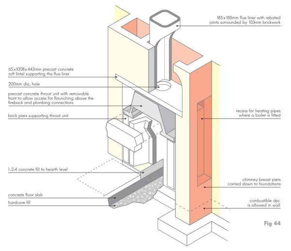
When an inset open fire is to be used the recess dimensions can be reduced by the introduction of two half-brick piers to support the precast concrete throat (Fig 44) unit which provides the necessary gather to the flue.
