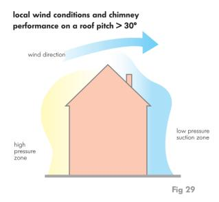
For a high pitched roof, (>30°,) the pressure on the windward side is greater than on its leeward side. See Fig. 29. A flue outlet located in this high pressure zone (Fig.30) may cause fume emission from an appliance it serves unless the outlet is raised above the high pressure zone or placed on the leeward slope in the suction zone.
