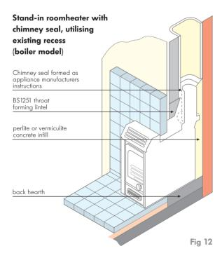
There are two types of roomheater. The 'dry' type and those with boilers which provide hot water for heating and domestic use. The boiler types have rated outputs from 3kW to 13kW.
