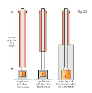
The main function of a chimney is to induce an adequate supply of combustion air and to remove the products of combustion produced by the appliance. Additionally the flue induces a flow of ventilation air which also assist in the prevention of condensation in the dwelling.
