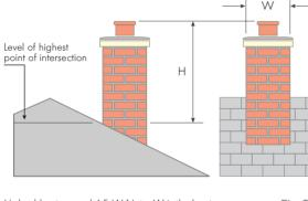
H should not exceed 4.5xW Note: W is the least horizontal dimension of the highest point of intersection with roof surface, gutter etc, and H is measured to top of any chimney pot or terminal Fig 25
