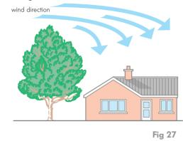
However well designed, constructed and positioned, the satisfactory performance of a flue can be adversely affected by downdraught caused by nearby hills, adjacent tall buildings or trees. These can deflect wind to blow directly down a flue or create a region of turbulence over the terminal.
