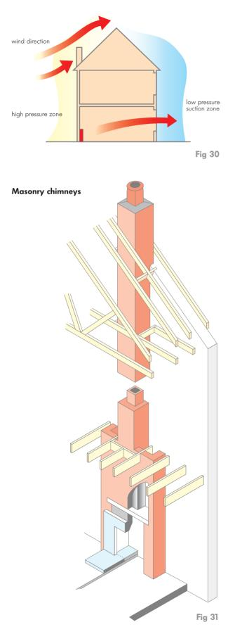
If the room in which the flue originates communicates by way of windows or other openings with the suction zone, (Fig 30) the possibility of appliance smoke emission will be increased.
