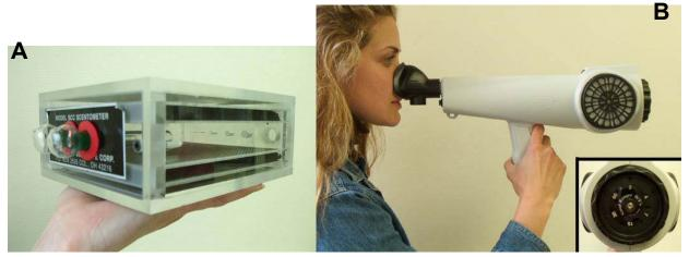
Figure 3. (A) The Scentometer Field Olfactometer (Barneby Sutcliffe Corp.). Note the two glass nostril ports to the left and the series of orifices at the back of the unit to the right of the photo. (B) The Nasal Ranger Field Olfactometer (St. Croix Sensory). The inset picture shows the orifice dial, which is located at the right side of the Nasal Ranger in this photo.
