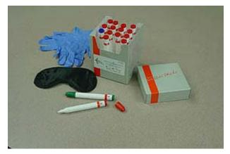
Figure 2. The St. Croix Sensory Odor Pen Testing Kit, manufactured by Burghart. Included in the kit are a blindfold, latex gloves, and the set of 14 odor pens (red) and two blank pens.
