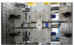
Fig. 3: 72+72-fold stack mold with 6 servo motors for closing cone
