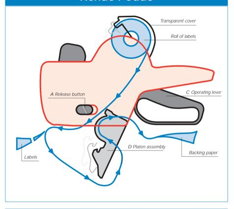
Lift transparent cover and place roll of labels into the machine.
