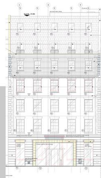
Office refurbishment for a leading finance company in central London, including total internal demolition and strip-out of an existing 4-storey office building with façade retention to front and rear, 2-storey extension and basement enlargement.
