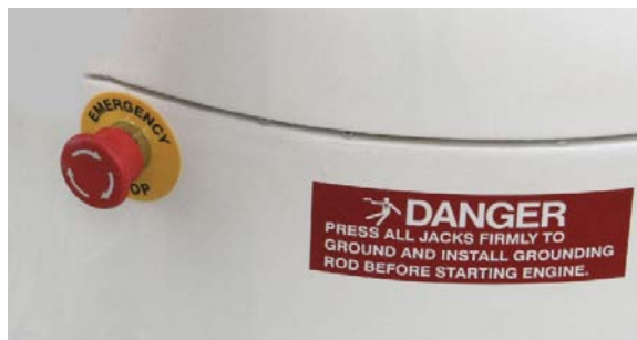
Fig 1-15 Emergency Stop button
