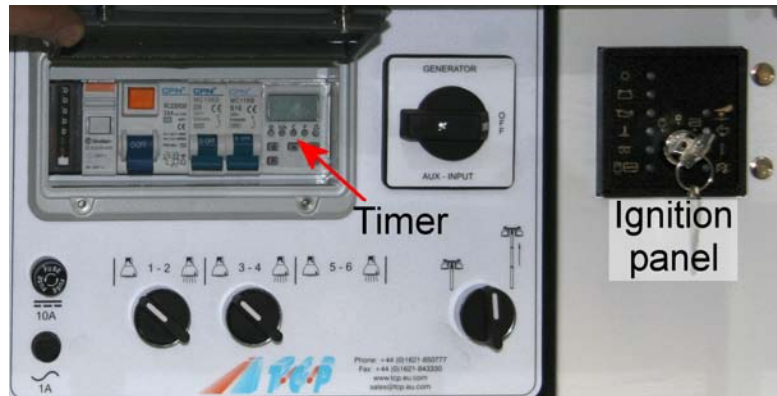
Fig A1 Timer and ignition panel
