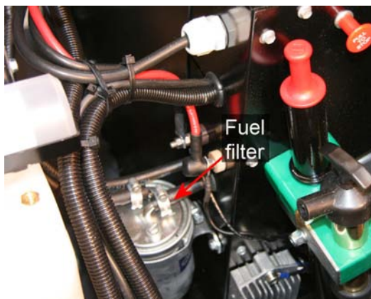
Fig 2-5 Fixed fuel filter
