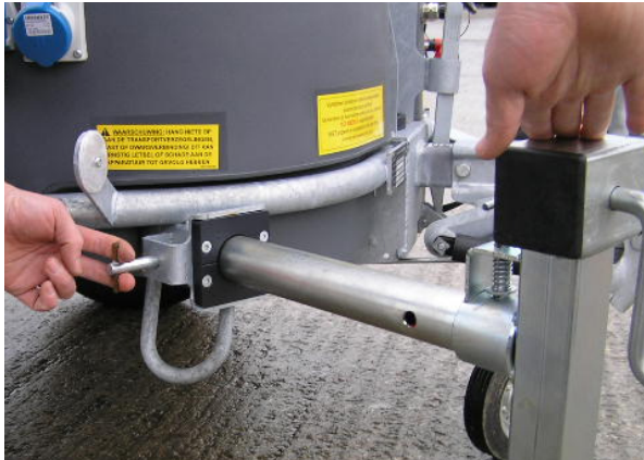
Fig 1-5 Extending the jack
