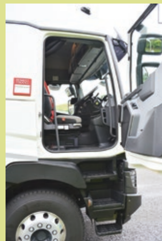
The three well placed access steps are complemented by generous grab handles.
