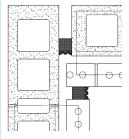
Seismic Colorseal is an excellent, simple sealing solution at inside corner conditions where it is impossible to install mechanically fastened 'strip-seal' systems. In cavity-wall conditions, installation of Seismic Colorseal in the structural backup maintains integrity of thermal insulation as well as the air barrier while preventing passage of cavity moisture into the structure.
