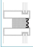
Seismic Colorseal is uniquely suited to sealing structural joints in curtain walls. Non-invasive anchoring means that mullions are not violated by screwing through them as occurs with "strip-seal" systems.
