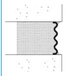
Seismic Colorseal is held in place by the backpressure of the expanding foam in conjunction with a field-installed bead of silicone caulk at the substrate-to-bellows interface.
